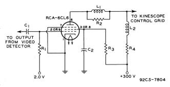
Fig. 1 - Typical Video Output Circuit Having Bandwidth of 4 Megacycles.
